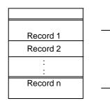
Figure 8.3: Structure of a cyclic file
