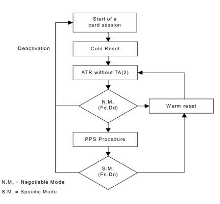
Figure I.1: Modes of operation of a "Type 1 UICC"
