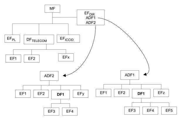
Figure 8.1: Example of an application structure
