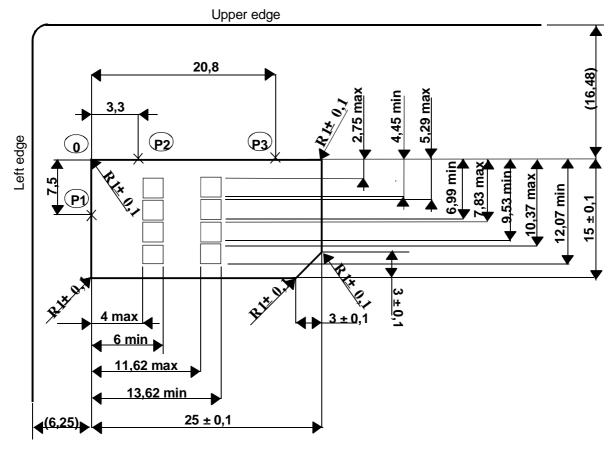
Figure 4.1: Plug-in UICC
