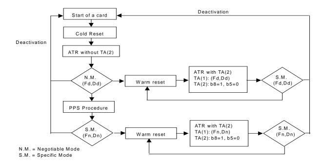
Figure I.2: Modes of operation of a "Type 2 UICC"
