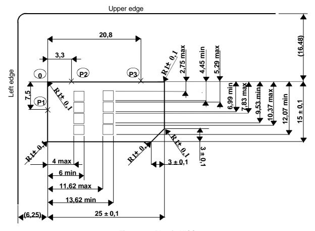
Figure 4.1: Plug-in UICC
