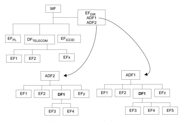
Figure 8.1: Example of an application structure
