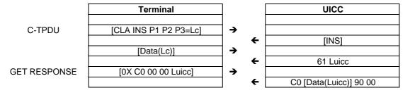
An R-APDU of {[Data(Luicc)] 90 00} is returned from the UICC to the terminal.
