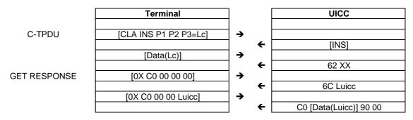
An R-APDU of  $\{[Data(Luicc)]\ 62\ XX\}$  is returned from the UICC to the terminal containing the data returned together with the warning status bytes.
