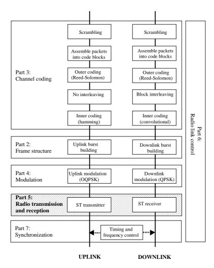
Figure 4: Physical layer functions
