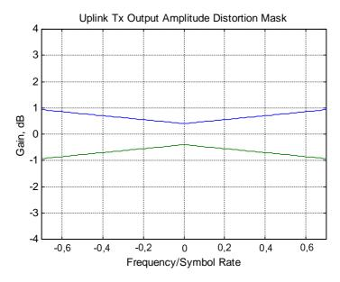
Figure 6.2.3: Uplink output amplitude non-linearity mask
