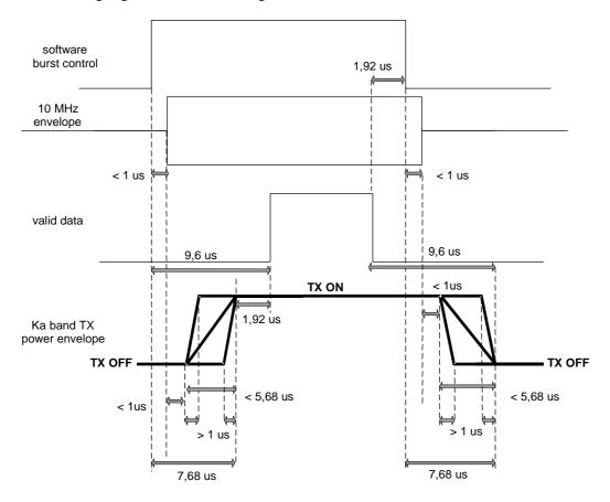
Figure 7.3: Ramp up and ramp down times
