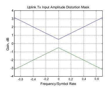
Figure 6.2.2: Uplink input amplitude non-linearity mask
