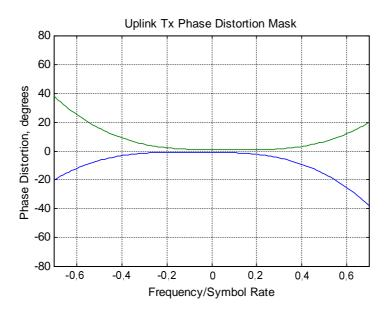
Figure 6.2.1: Uplink input phase non-linearity mask
