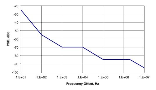
Figure 6.2.5: ST Uplink Phase Noise Mask
