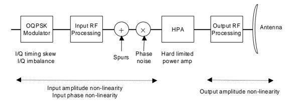
Figure 6.2: Uplink signal reference model
