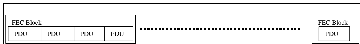
Figure 33: Downlink TDMA payload structure
