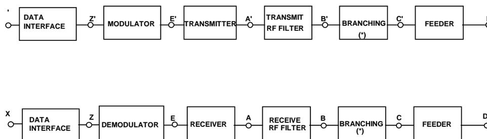
NOTE 1: For the purpose of defining the measurement points, the branching network does not include a hybrid.
