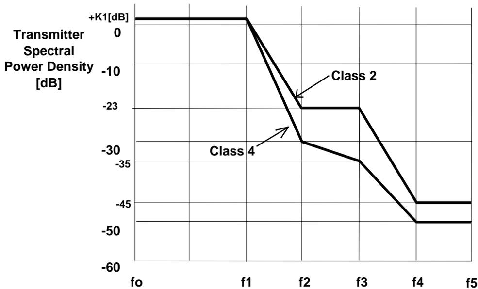
NOTE: Frequency from actual transmitter centre frequency [MHz].
