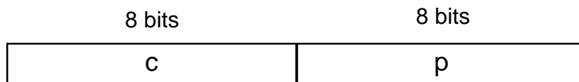
Figure 19: Data structure of the transmitter identification Information carried in the TII sub-fields
