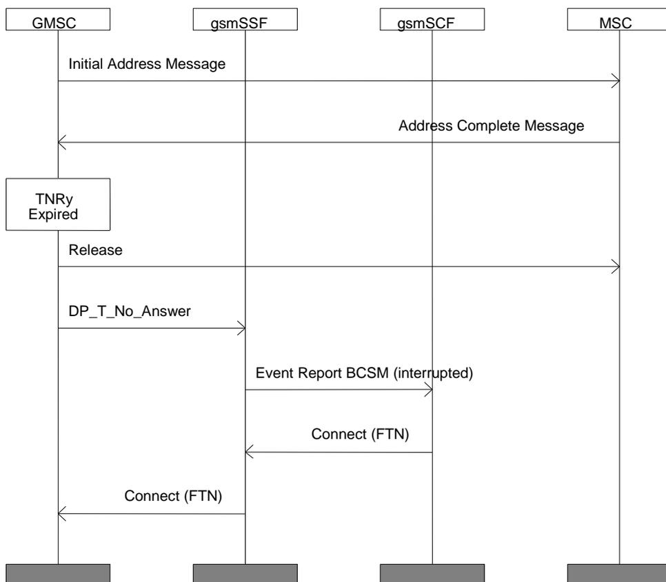
NOTE: The timer TNRy is started in the GMSC after the Address Complete Message has been received from the destination exchange. If this timer expires before an Answer message is received from the destination exchange, a release message is sent to the destination exchange and the detection point T\_No\_Answer is reached. This is specified in GSM 03.18 and GSM 03.78.
