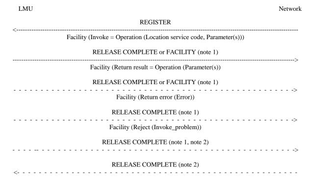
NOTE 1: If the network initiated operation does not require a result, reject or error to be returned then the LMU may release the transaction by sending a RELEASE COMPLETE message without a Facility Information Element and release of transaction by LMU is allowed (i.e. Release Forbidden has not been present in Register message). If release is not allowed by LMU, the LMU sends the result using Facility message.
