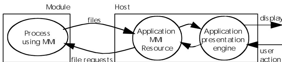
**Figure 17: Overview of the operation of an Application MMI resource**
