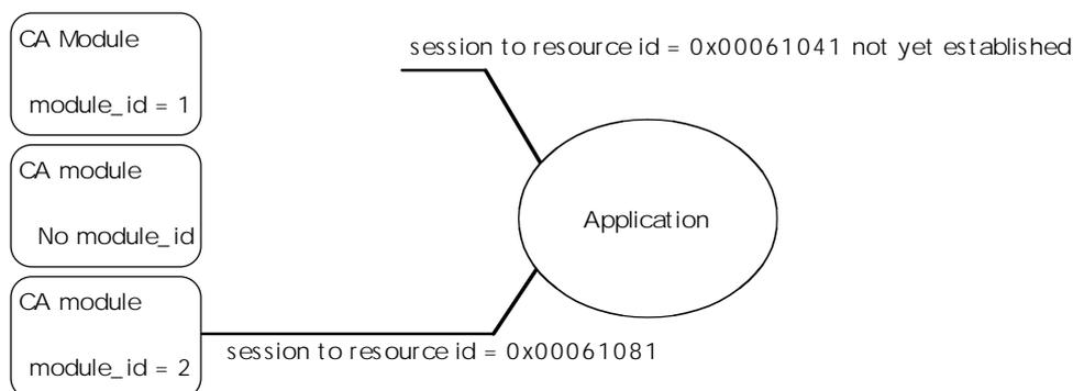
Figure 21: Use of module IDs to discriminate CAP resource instances
