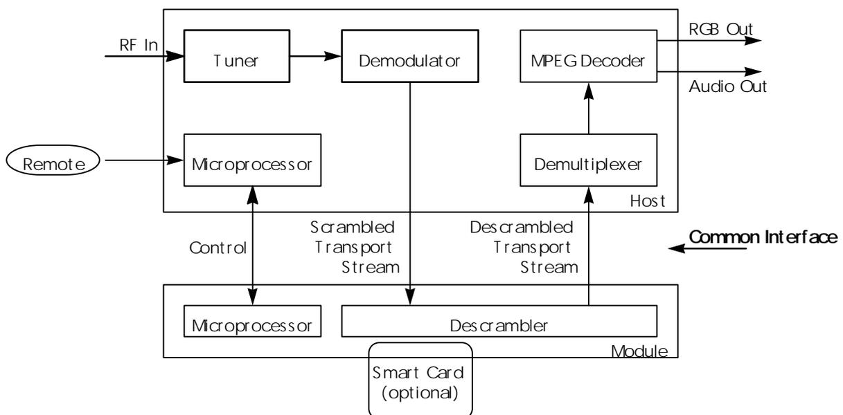
**Figure 1: Example of single module in connection with host**
