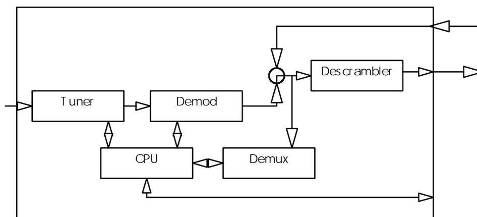
**Figure 7: Type 'B' input module with CA**
