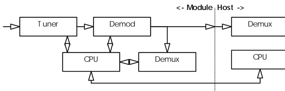
**Figure 6: Illustrative type 'B' module for broadcast networks**
