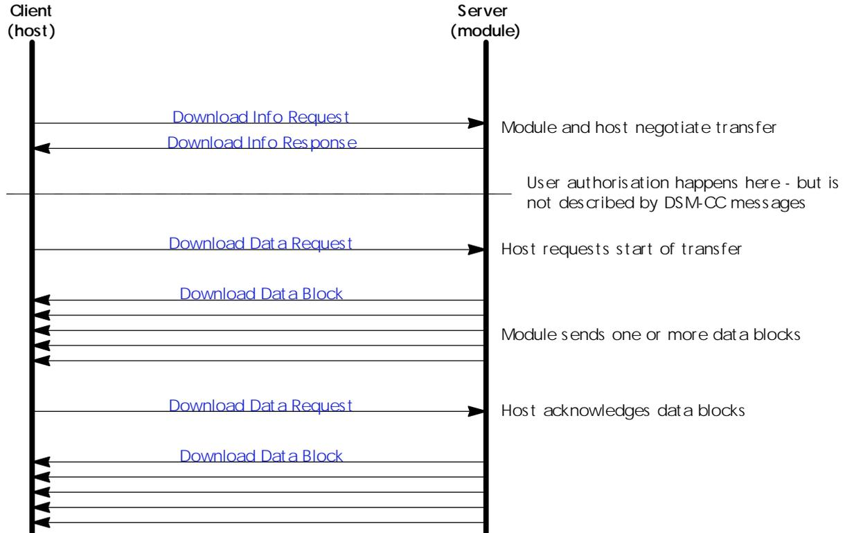
**Figure 19: DSM-CC Client - Server messages**
