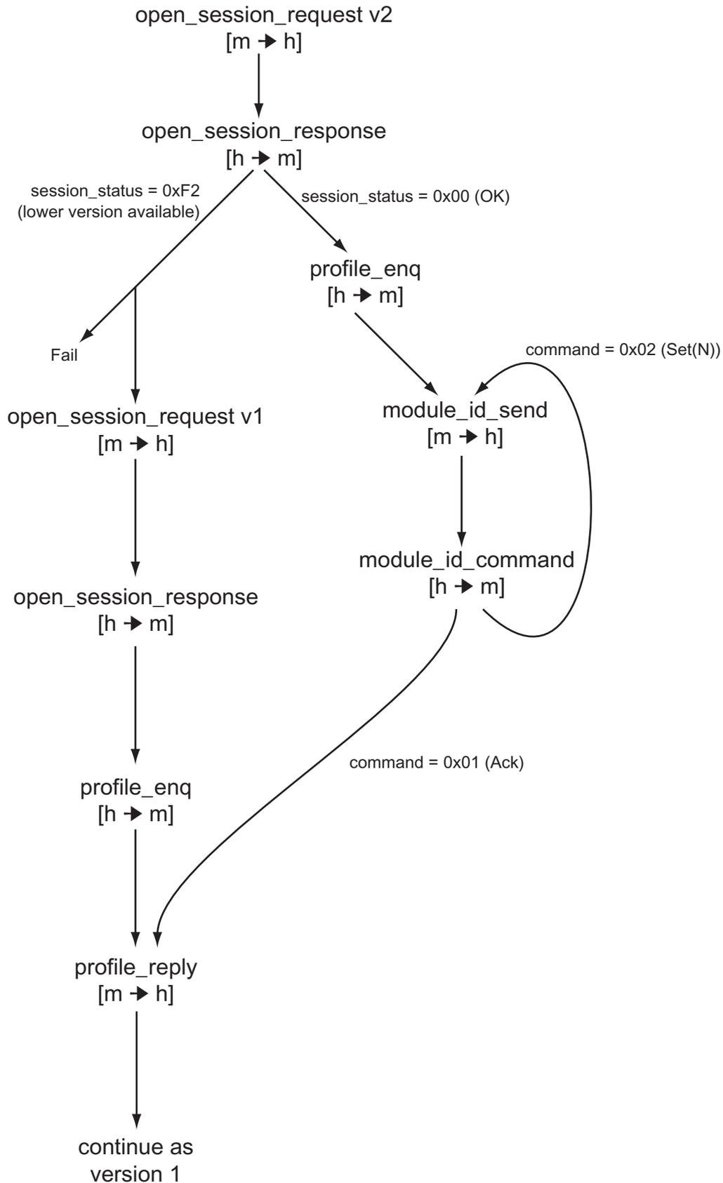
Figure 3: Module ID establishment
