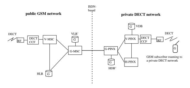
Figure 2a: End-to-end Interworking Reference Configuration - Scenario 2a
