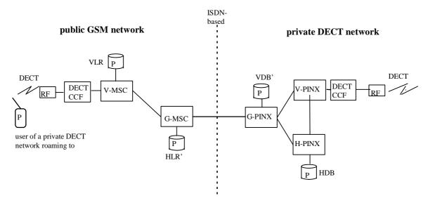
Figure 2b: End-to-end Interworking Reference Configuration - Scenario 2b
