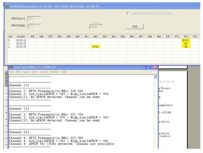
Figure B.6: Detection with GSM-R power level of -80 dBm, TX4 not available
