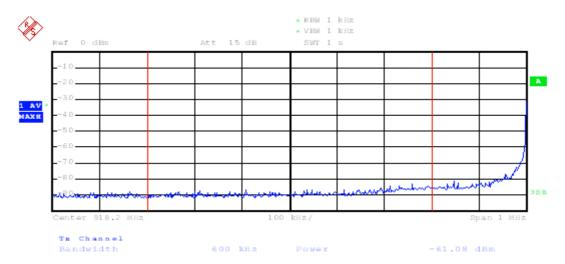
Figure A.13: Channel Power of the lower sideband without tag in the antenna field
