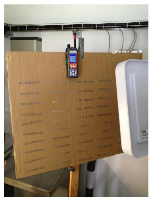
Figure B.10: GSM-R mobile placed opposite of the demonstrator and just above the RFID tags
