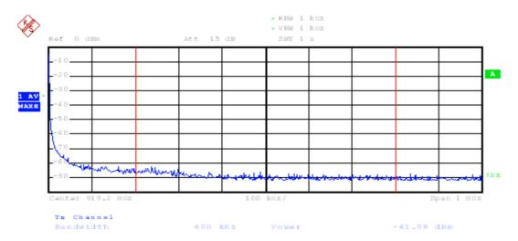
Figure A.11: Channel power of the upper sideband without tag in the antenna field
