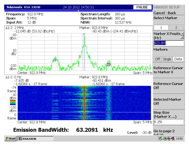
Figure C.7: Measured spectrum at test site with  $f_{GSM-R,second} = 921,8 \text{ MHz}, f_{TX4} = 922,9 \text{ MHz}, f_{GSM-R,first} = 923,8 \text{ MHz}$
