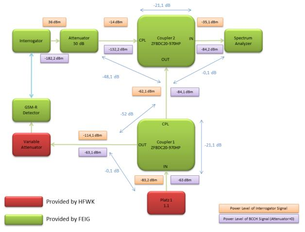
Figure 9 shows the test setup for detection tests.
