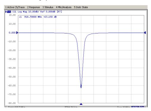
Figures A.5 and A.6 show the filtering capabilities of the notch filter.
