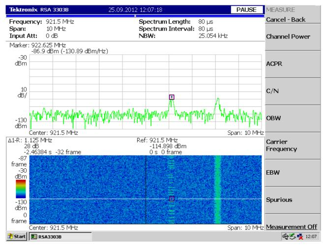
Figure B.5: All channels disabled. Only first and second GSM-R carriers are visible at  $f_{GSM-R,first} = 924,6 \text{ MHz}$  and  $f_{GSM-R,second} = 922,6 \text{ MHz}$
