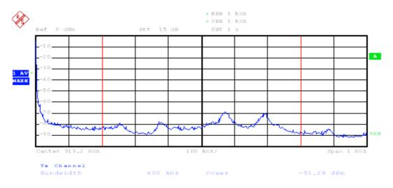
Figure A.10: Channel Power of the upper sideband with tag in the antenna field
