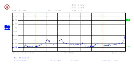
Figure A.12: Channel power of the lower sideband with tag in the antenna field
