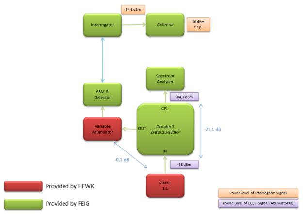
Figure 8: Performance test setup
