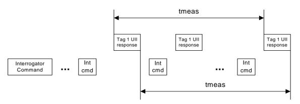
Figure 11: Illustration for time to be measured
