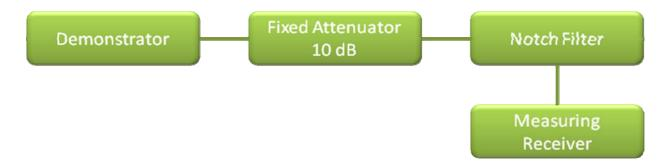
Figure A.4: Test Setup with Notch Filter for Measurement of the Transmitter Spectrum Mask
