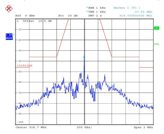
Figure A.7 shows the spectrum of the demonstrator with the additional notch filter inserted into the test setup.
