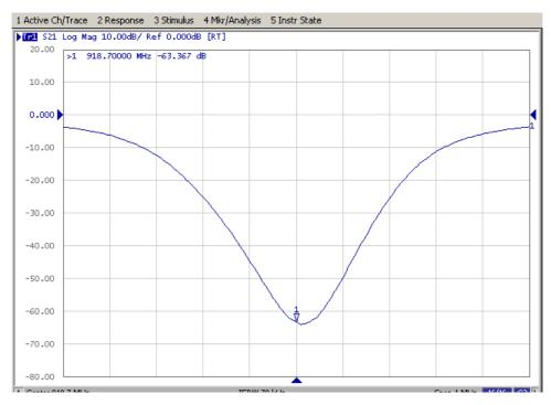
Figure A.6: S21 of the Notch Filter measured with a Network Analyser, Span 1 MHz
