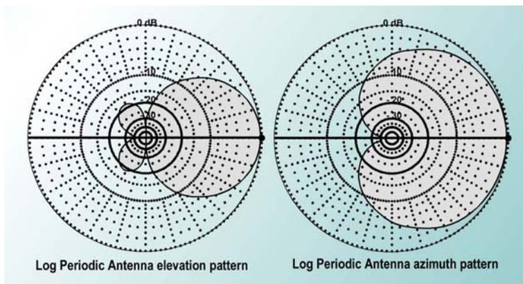
Figure 2: Sample Antenna Directional Pattern
