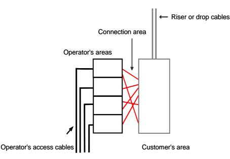
Figure 3: Illustration of a Distribution Point
