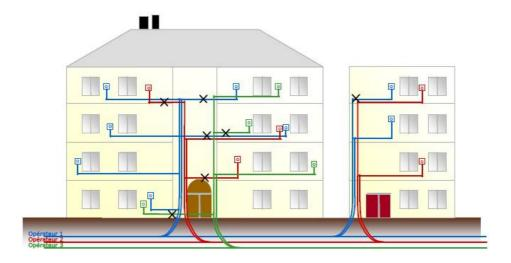
Figure 1: Individual building cabling for each operator
