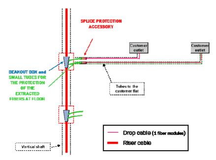
Figure 5: Example of a Distribution System
