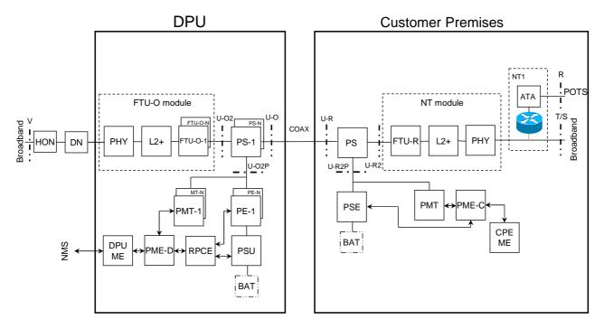
Figure 4: RPFA-CGO Reference Model with a single derived POTS port
