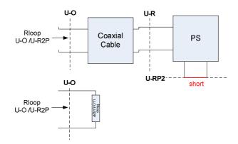
Figure 10: Loop resistance U-R2P to U-O interface
