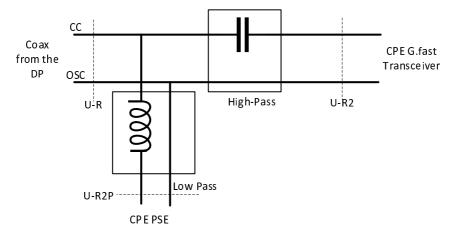
Figure 13: CPE Power Splitter for RPFA-CGO and RPFA-CGS
