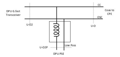
Figure 14: DPU Power Splitter for RPFA-CGO and RPFA-CGS
