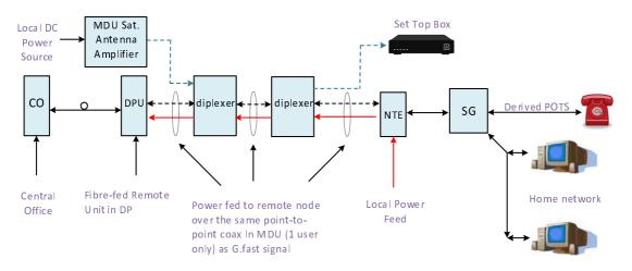
Figure 1: Generic Fibre-fed Remote Node Coaxial Architecture with Reverse Power Feed
