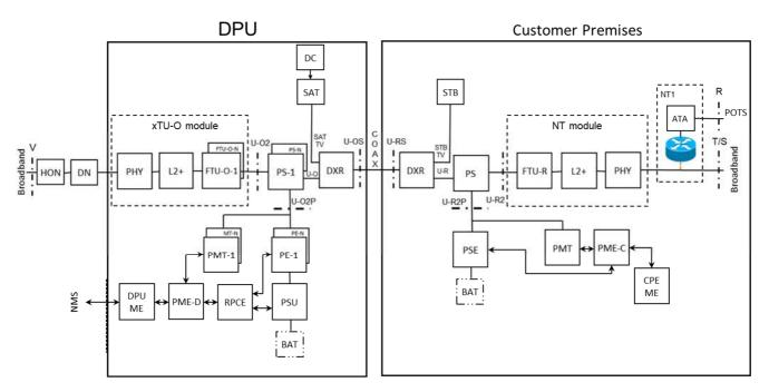
Figure 6: RPFA-CGS Reference Model with a single derived POTS port
