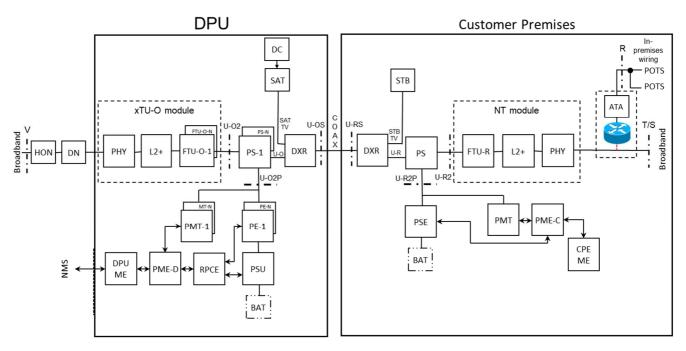
Figure 7: RPFA-CGS Reference Model with a derived POTS port distributed over In-premises wiring
