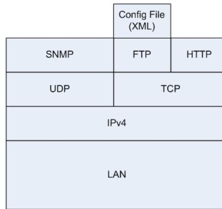
**Figure 8.6: Protocol Stack for RCST management from the LAN interface**
