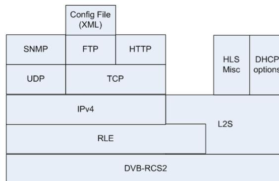
**Figure 8.7: Protocol Stack for RCST satellite interface management (return link)**
