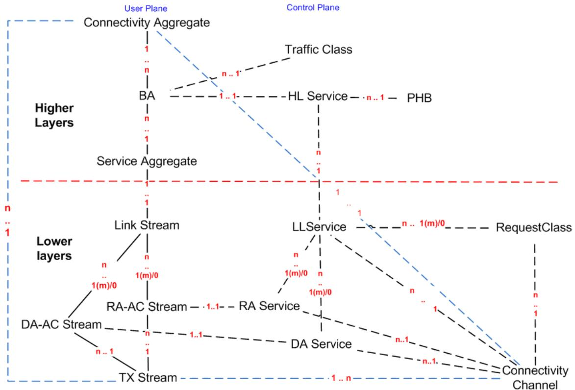
**Figure 7.5: RCST QoS Control and Traffic model**
