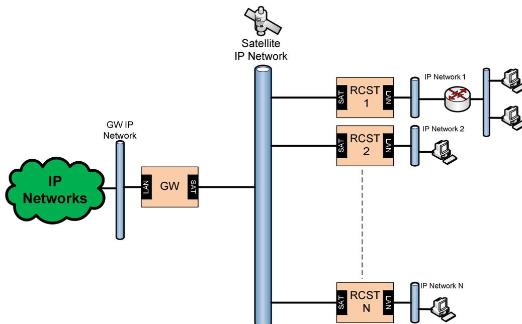
Figure 7.2: Example routing topology for a GW connecting N RCSTs
