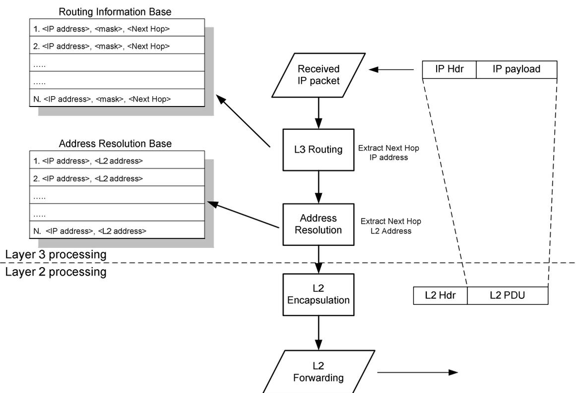
**Figure 7.1: RCST Unicast IP packet forwarding**
