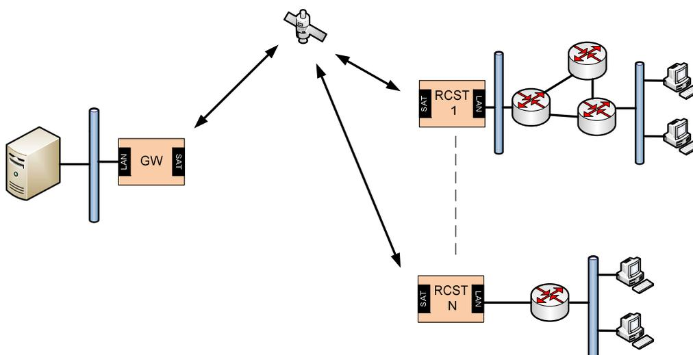
Figure 7.3: Multiple networks connected to an RCST
