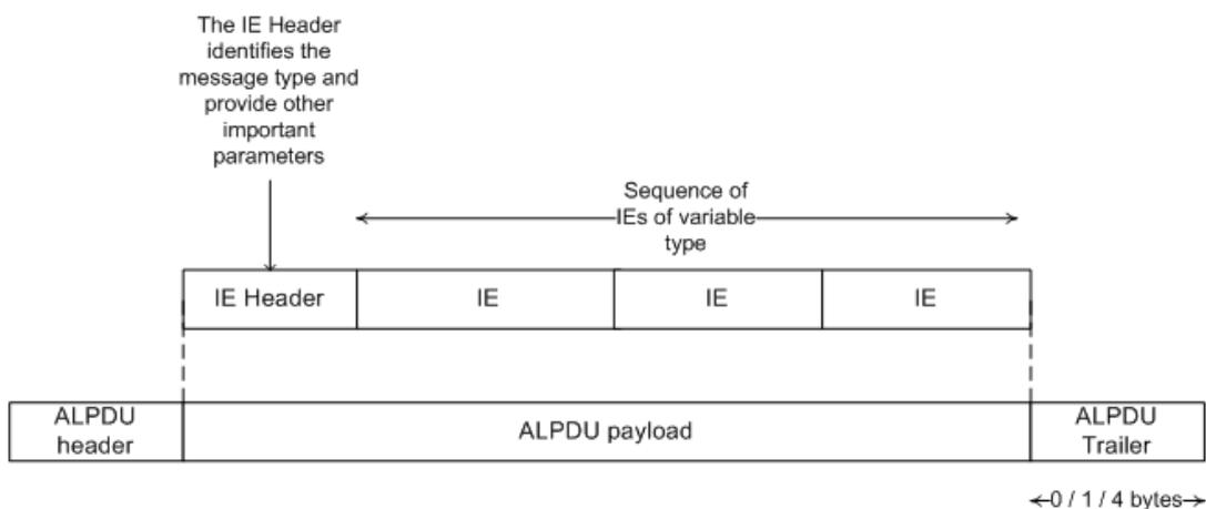
**Figure D.2: DCP messages structure over L2**
