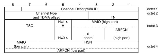
Figure 10.5.2.5a.1/3GPP TS 04.18: Channel Description 2 information element
