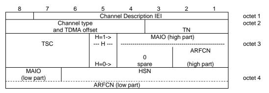
Figure 10.5.2.5.1/3GPP TS 04.18: Channel Description information element
