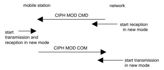
Figure 3.4.7.2.1/3GPP TS 04.18: Ciphering mode setting sequence
