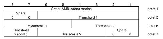
Figure 10.5.2.21aa.4/3GPP TS 04.18: Parameters for multirate speech field for the MR version 1 when a set of three codec modes is chosen
