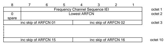
Figure 10.5.2.12.1/3GPP TS 04.18: Frequency Channel Sequence information element
