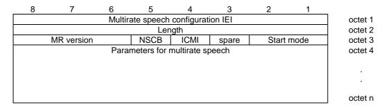
Figure 10.5.2.21aa.1/3GPP TS 04.18: MultiRate configuration information element
