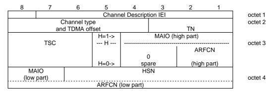
Figure 10.5.2.5.1/3GPP TS 04.18: Channel Description information element
