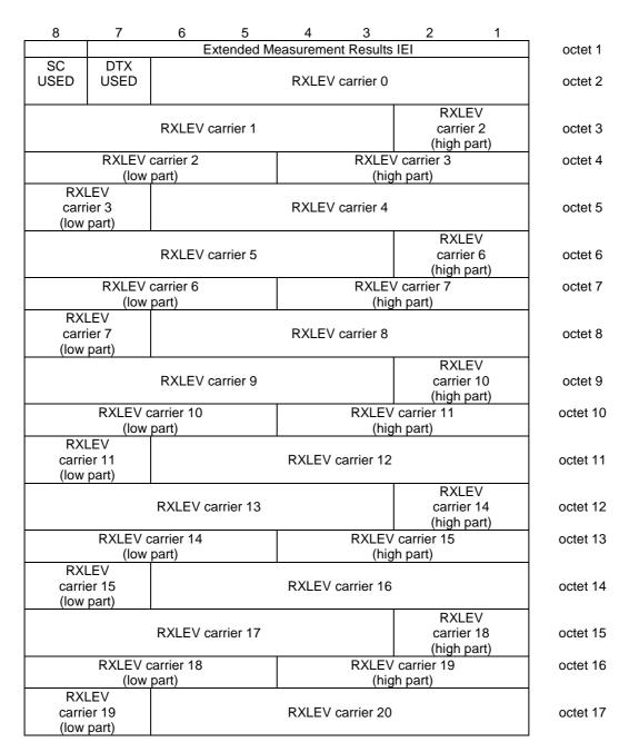
Figure 10.5.2.45.1/3GPP TS 04.18: Extended Measurement Results information element
