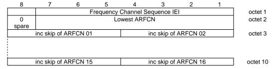
Figure 10.5.2.12.1/3GPP TS 04.18: Frequency Channel Sequence information element
