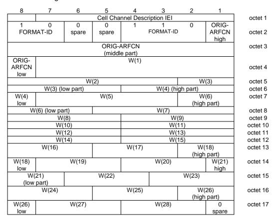
Figure 10.5.2.1b.6.1//3GPP TS 04.18: Cell Channel Description information element, range 128 format
