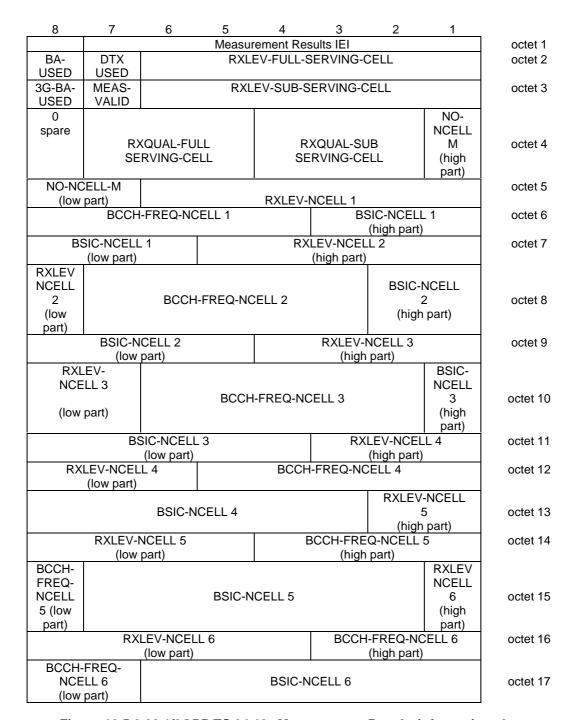
Figure 10.5.2.20.1/3GPP TS 04.18: Measurement Results information element
