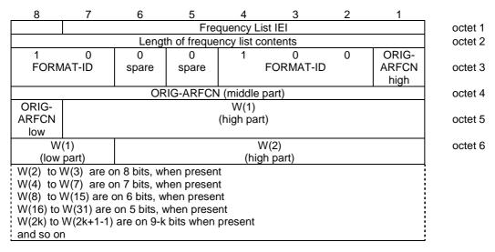
Figure 10.5.2.13.4.1/3GPP TS 04.18: Frequency List information element (Range 512 format)
