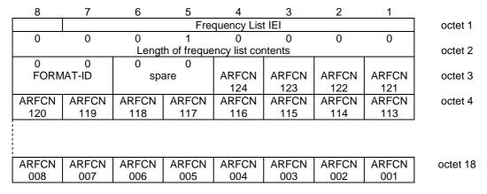
Figure 10.5.2.13.2.1/3GPP TS 04.18: Frequency List information element, bit map 0 format
