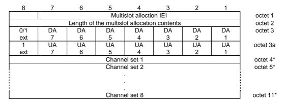
Figure 10.5.2.21b.1/3GPP TS 04.18: Multislot Allocation information element
