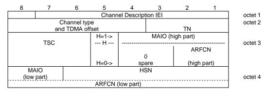
Figure 10.5.2.5a.1/3GPP TS 04.18: Channel Description 2 information element
