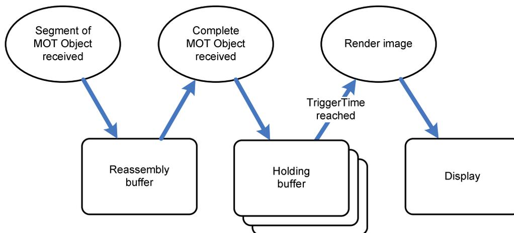
**Figure 5.2: Enhanced profile Buffer management model for a MOT SlideShow decoder**
