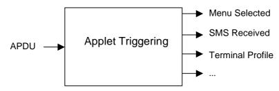
Figure 3: toolkit applet triggering diagram
