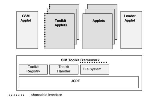
Figure 1: GSM Java Card Architecture
