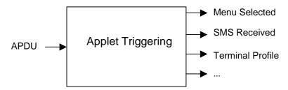
Figure 3: toolkit applet triggering diagram
