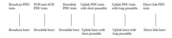
Independently of the burst type each burst consists of two sections: preamble and payload. Each burst is started with a preamble section,  $r_{PAYLOAD}$ , which is followed by a payload section,  $r_{PAYLOAD}$ , and its baseband format is
