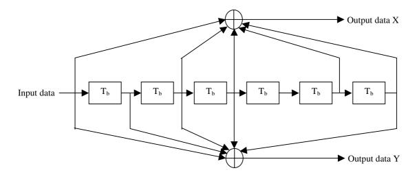
Figure 4: The mother convolutional code of rate 1/2
