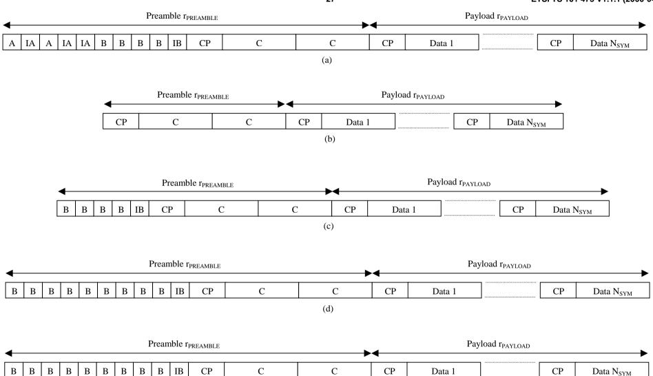
Figure 17: PHY burst structures: (a) Broadcast burst, (b) Downlink burst, (c) Uplink burst with short preamble, (d) Uplink burst with long preamble, (e)
