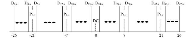
Figure 9: Sub-carrier frequency allocation
