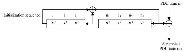
Figure 2: Scrambler schematic diagram
