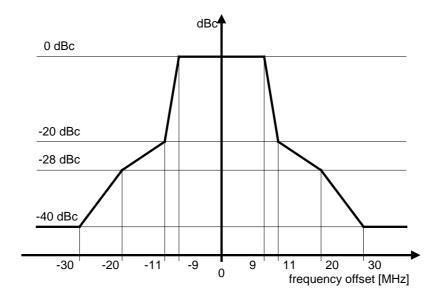
Figure 18: Transmit spectral power mask. dBc is the spectral density relative to the maximum spectral power density of the transmitted signal
