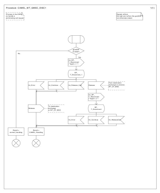
Figure 26a: Procedure CAMEL\_MT\_GMSC\_DISC1 (sheet 1)
