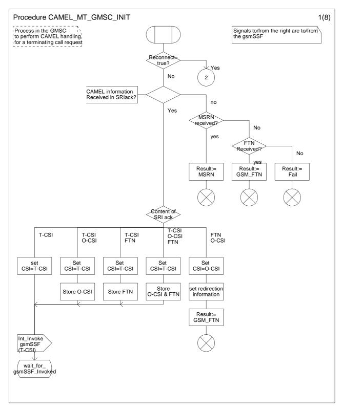
Figure 24a: Procedure CAMEL\_MT\_GMSC\_INIT (sheet 1)
