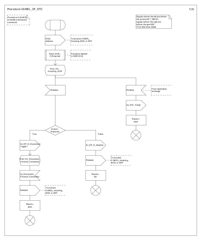
Figure 41a: Process CAMEL\_CF\_ETC (sheet 1)
