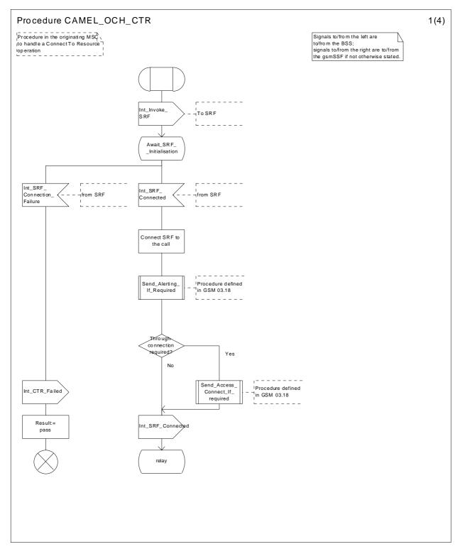
Figure 18a: Procedure CAMEL\_OCH\_CTR (sheet 1)
