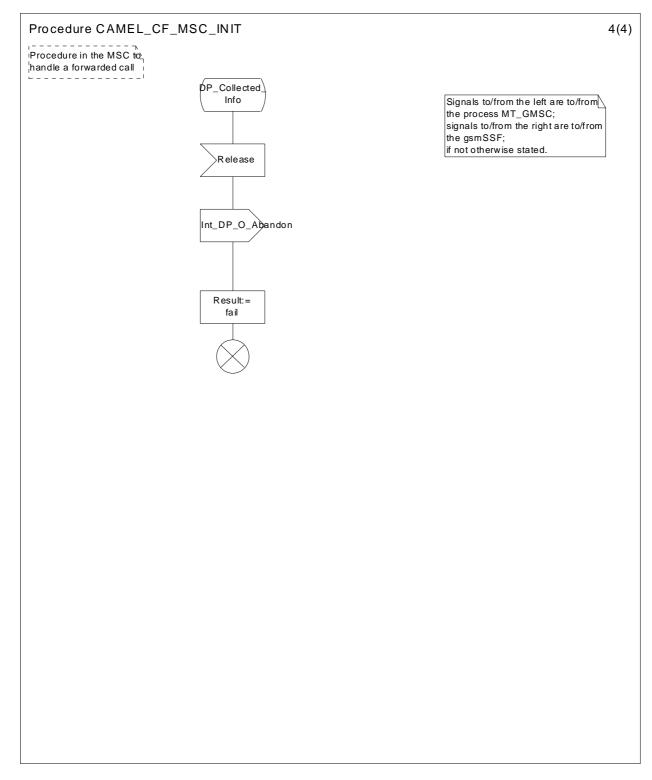
Figure 39d: Procedure CAMEL\_CF\_MSC\_INIT (sheet 4)
