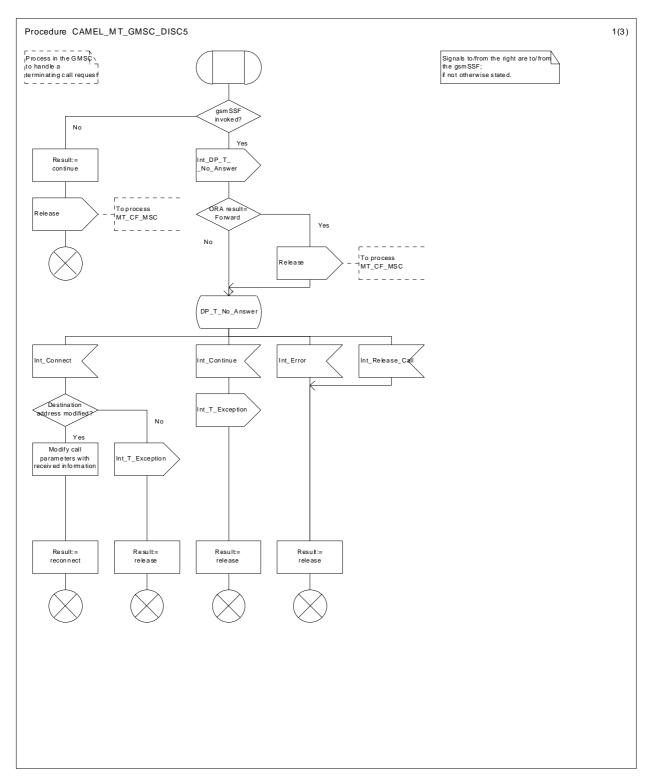
Figure 29a: Procedure CAMEL\_MT\_GMSC\_DISC5 (sheet 1)
