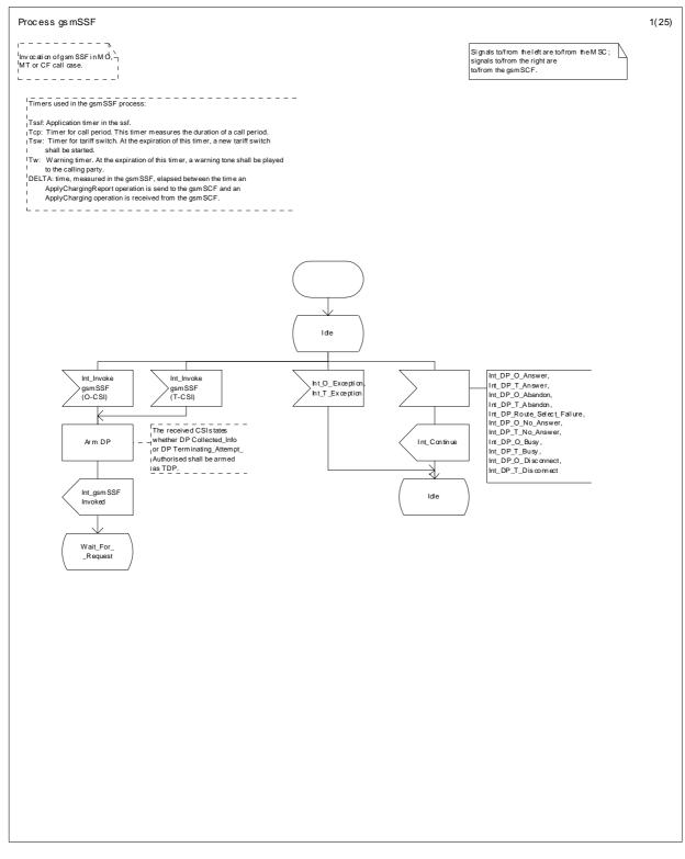
Figure 45a: Process gsmSSF (sheet 1)
