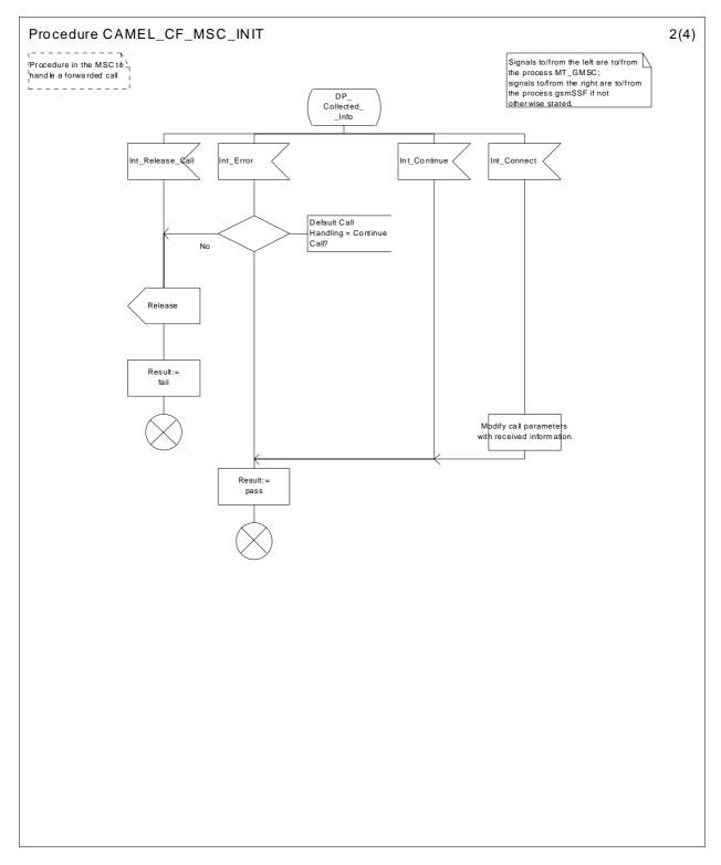
Figure 39b: Procedure CAMEL\_CF\_MSC\_INIT (sheet 2)
