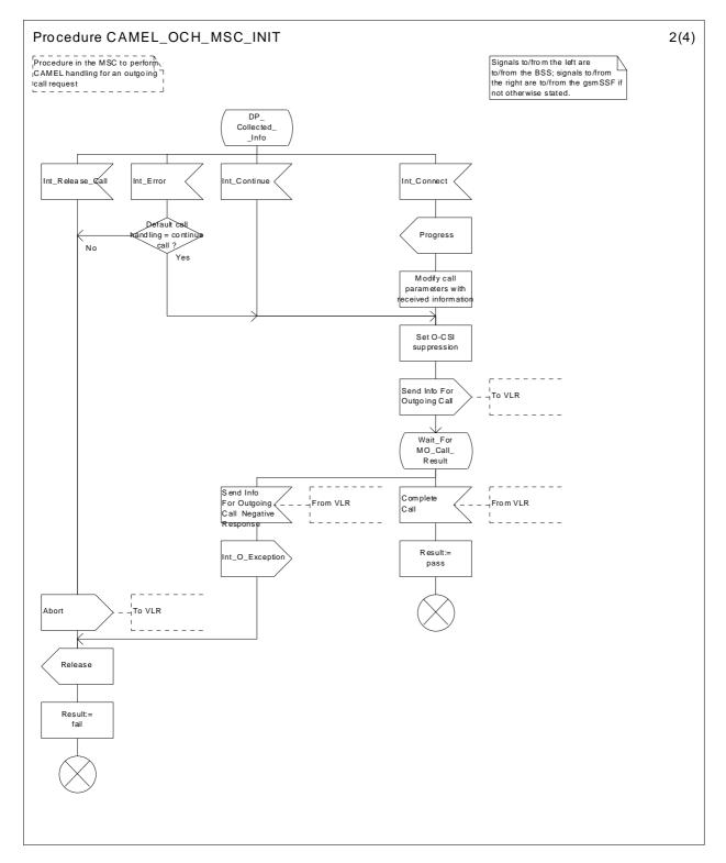
Figure 10b: Procedure CAMEL\_OCH\_MSC\_INIT (sheet 2)
