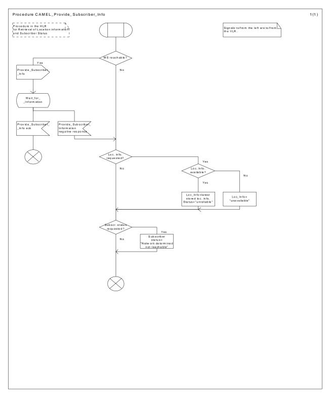
Figure 55a: Procedure CAMEL\_Provide\_Subscriber\_Info (sheet 1)
