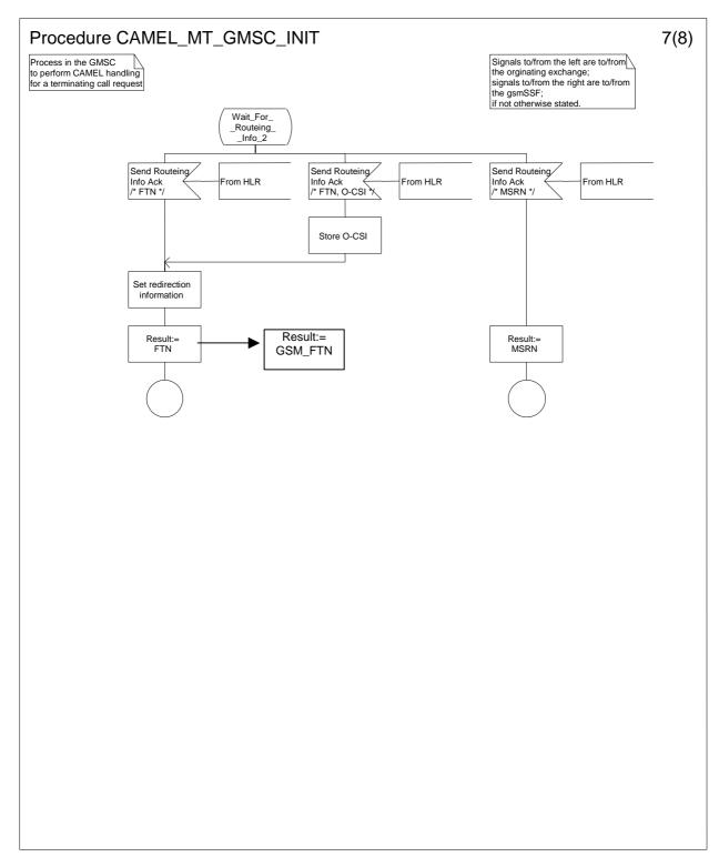
Figure 24g: Procedure CAMEL\_MT\_GMSC\_INIT (sheet 7)
