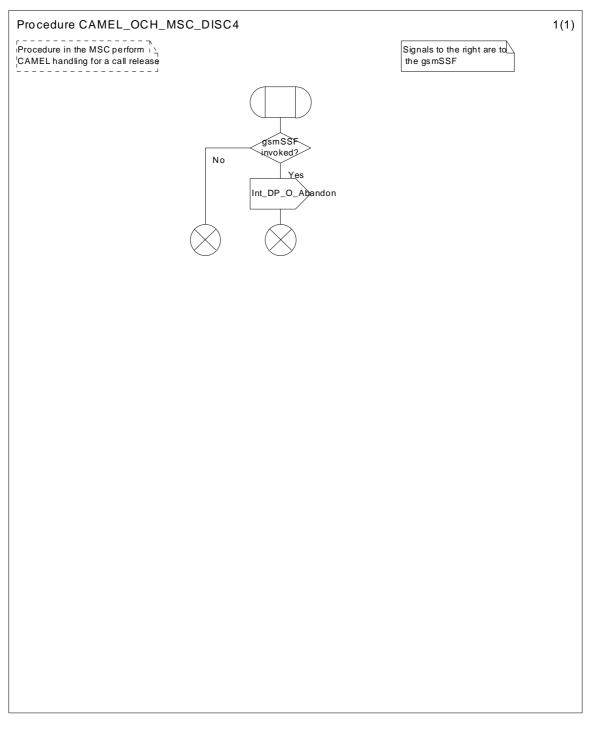
Figure 16a: Procedure CAMEL\_OCH\_MSC\_DISC4 (sheet 1)
