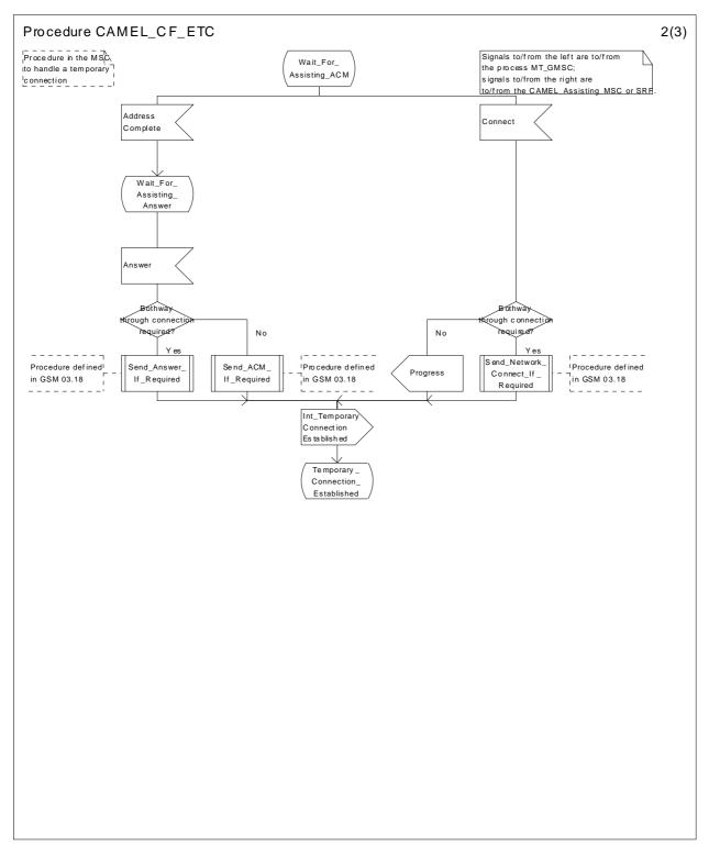
Figure 41b: Procedure CAMEL\_CF\_ETC (sheet 2)
