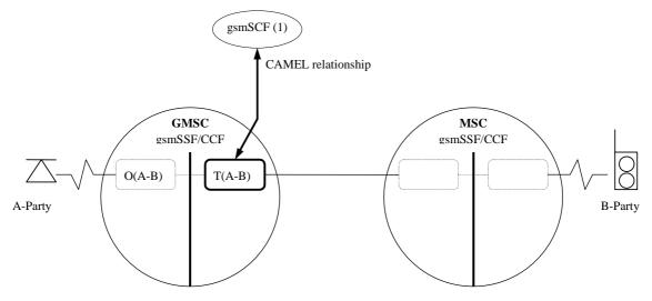
Figure 6: BCSM Scenario for Mobile Terminated Calls
