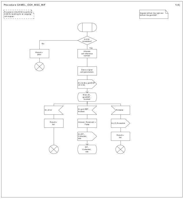
Figure 10a: Procedure CAMEL\_OCH\_MSC\_INIT (sheet 1)
