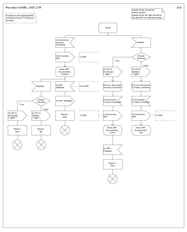
Figure 18b: Procedure CAMEL\_OCH\_CTR (sheet 2)
