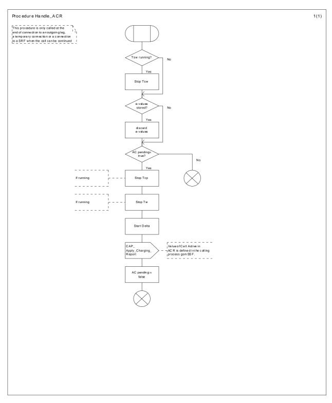
Figure 48a: Procedure Handle\_ACR (sheet 1)
