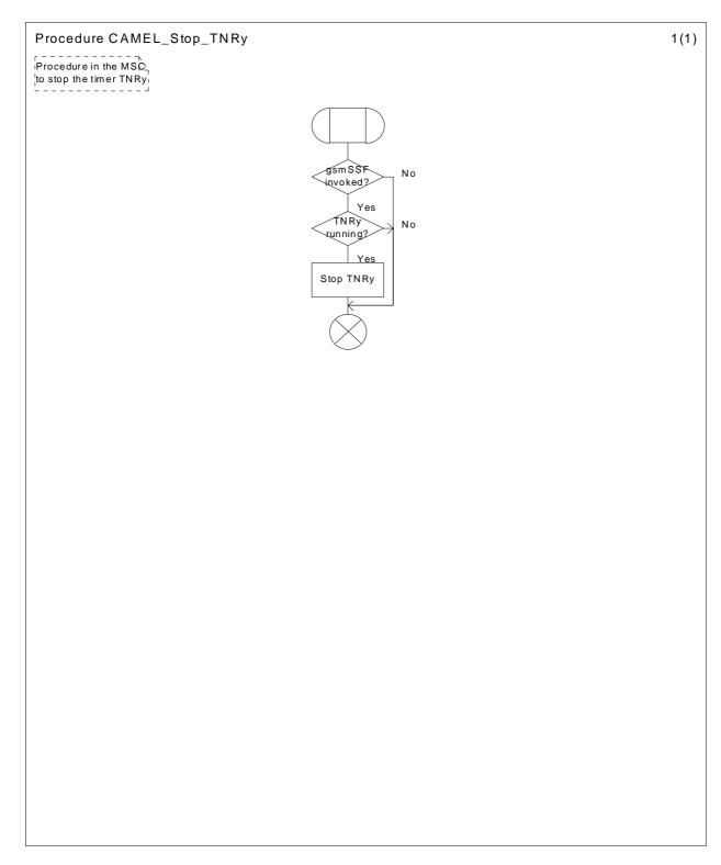
Figure 20a: Procedure CAMEL\_Stop\_TNRy (sheet 1)
