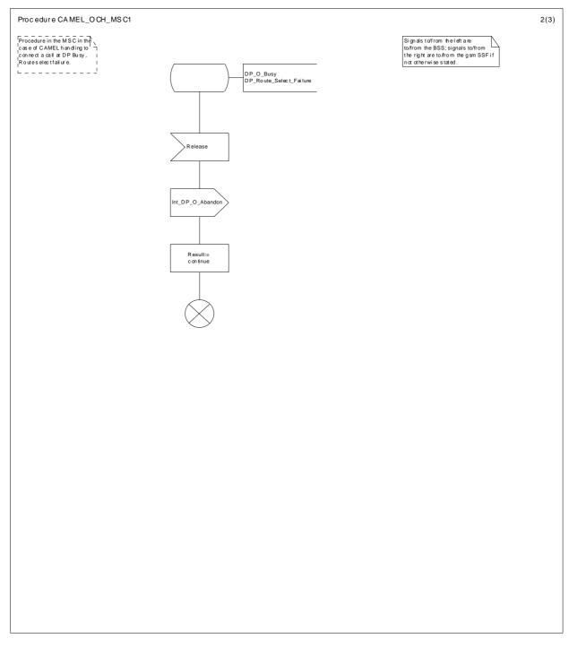
Figure 12b: Procedure CAMEL\_OCH\_MSC1 (sheet 2)
