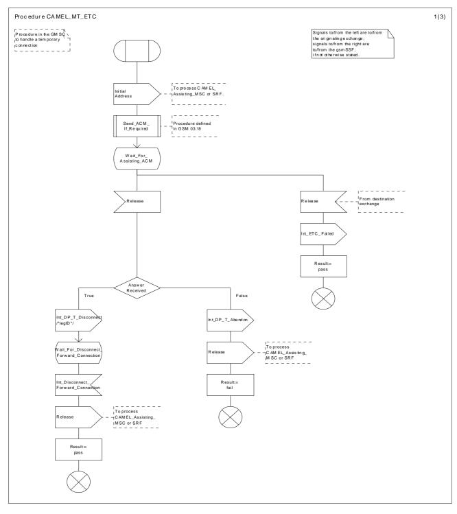
Figure 31a: Procedure CAMEL\_MT\_ETC (sheet 1)
