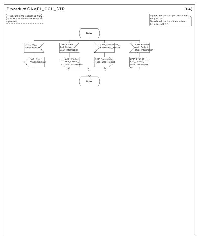
Figure 18c: Procedure CAMEL\_OCH\_CTR (sheet 3)
