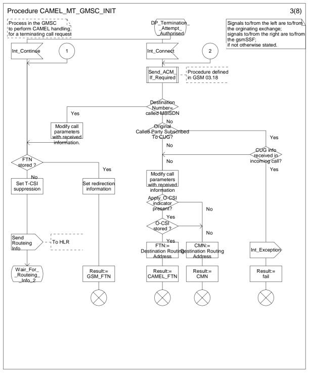
Figure 24c: Procedure CAMEL\_MT\_GMSC\_INIT (sheet 3)
