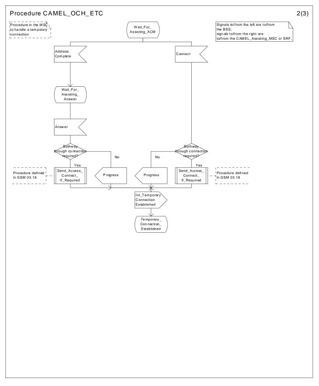
Figure 17b: Procedure CAMEL\_OCH\_ETC (sheet 2)
