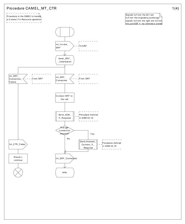
Figure 32a: Procedure CAMEL\_MT\_CTR (sheet 1)
