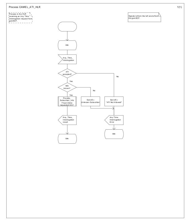
Figure 56a: Process CAMEL\_ATI\_HLR (sheet 1)
