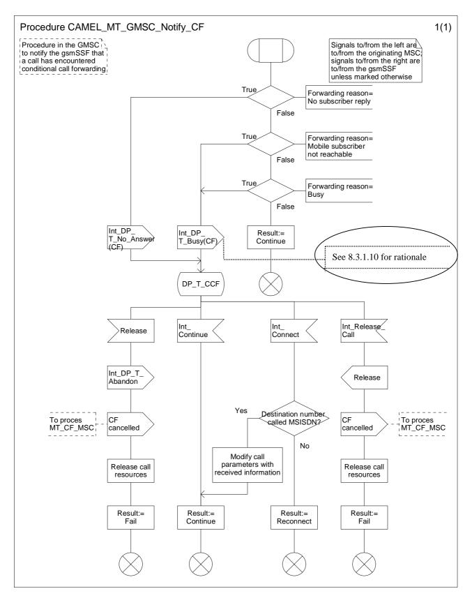
Figure 33a: Procedure CAMEL\_MT\_GMSC\_Notify\_CF (sheet 1)
