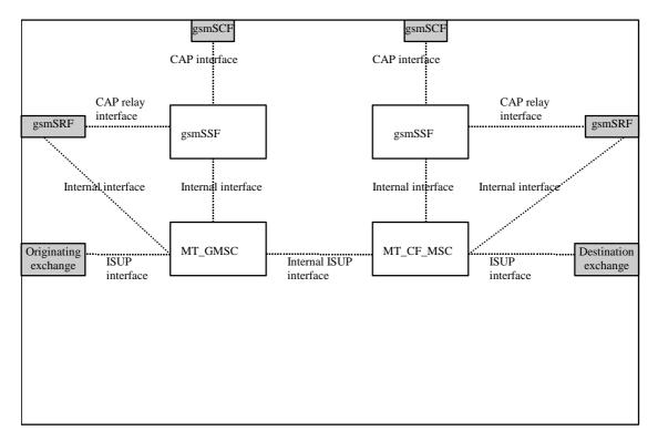
Figure 9c: Terminating case (gsmSSF relay)
