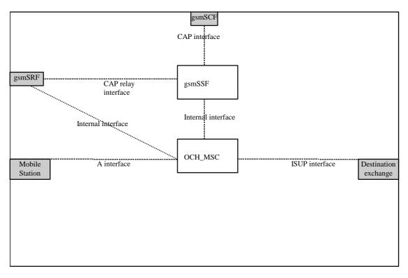
Figure 9a: Outgoing case (gsmSSF relay)
