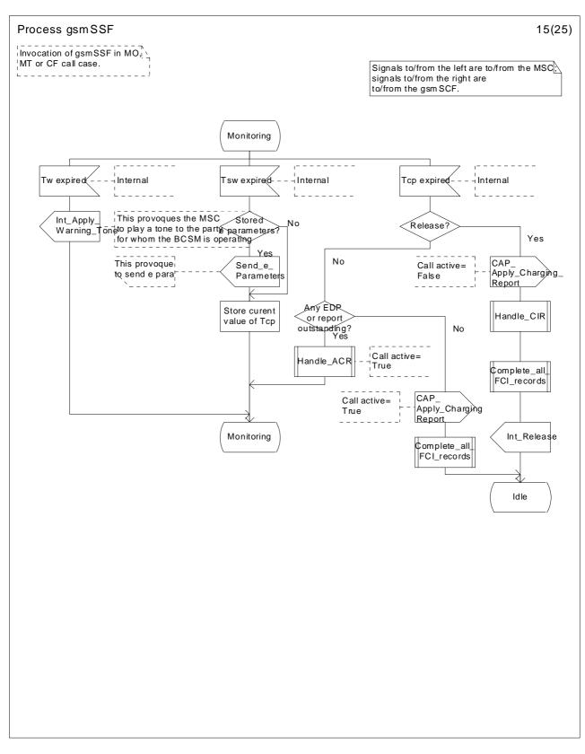
Figure 45n: Process gsmSSF (sheet 15)
