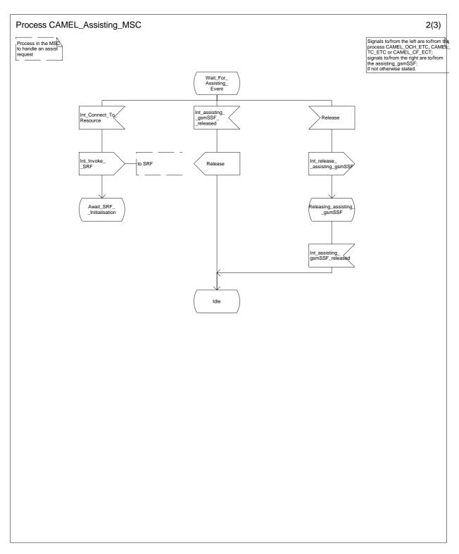
Figure 53b: Process CAMEL\_Assisting\_MSC (sheet 2)
