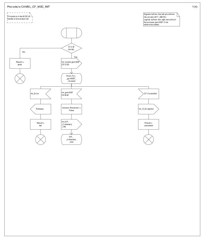
Figure 39a: Procedure CAMEL\_CF\_MSC\_INIT (sheet 1)
