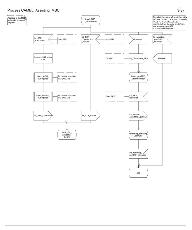
Figure 53c: Process CAMEL\_Assisting\_MSC (sheet 3)
