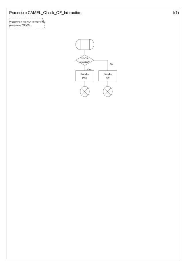
Figure 58a: Procedure CAMEL\_Check\_CF\_Interaction (sheet 1)
