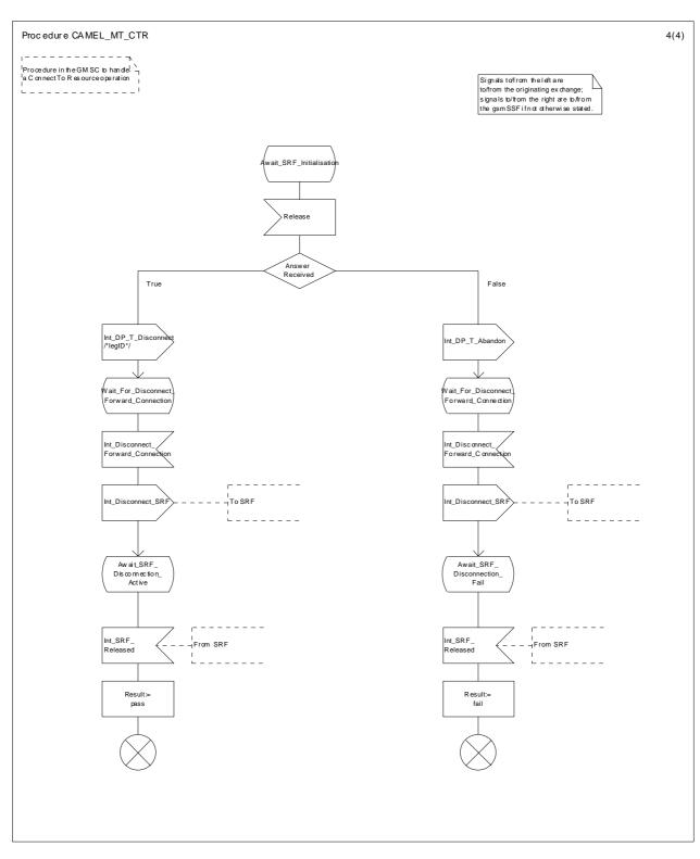
Figure 32d: Procedure CAMEL\_MT\_CTR (sheet 4)
