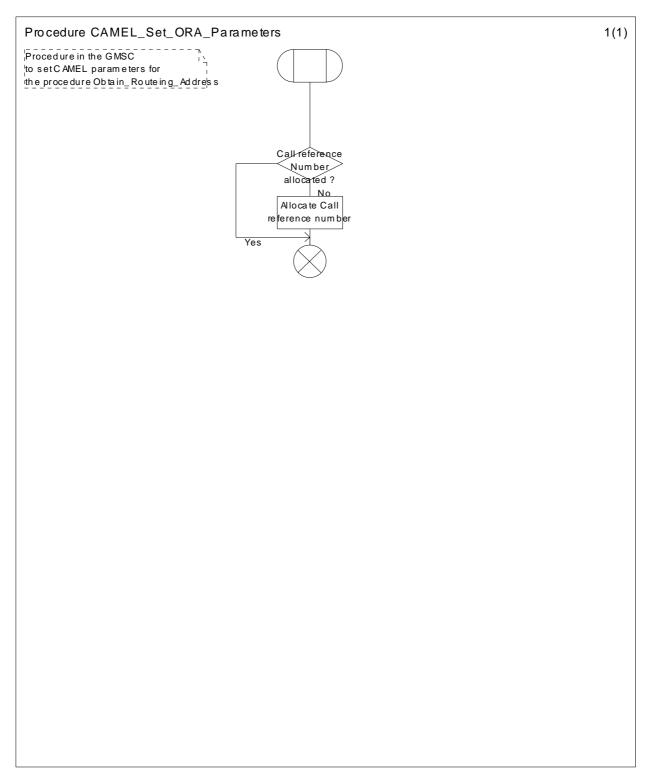
Figure 23a: Procedure CAMEL\_Set\_ORA\_Parameters (sheet 1)
