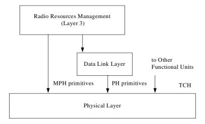
Figure 4.1: Interfaces with the physical layer
