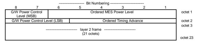
Figure 9.1.1: S-SACCH forward block format
