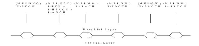
Figure 5.1.2: SAPs between the physical layer and the data link layer in the MES
