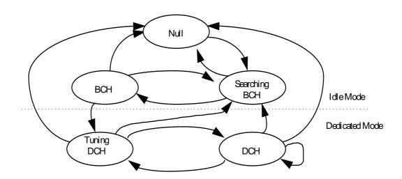
Figure 7.1: States of the physical layer in the MES
