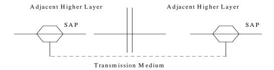
Figure 5.1.1: Service access point concept
