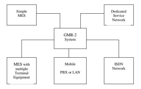
Figure 5.1: Examples of GMR-2 interfaces
