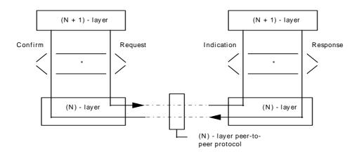
Figure 9.4.1: Primitive action sequence for peer-to-peer communication
