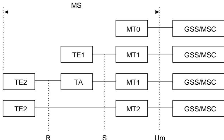
**Figure 1: GMR-1 Satellite System Access Reference Configuration**
