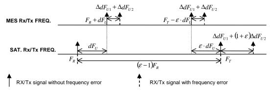
Figure 6.2: In call frequency correction
