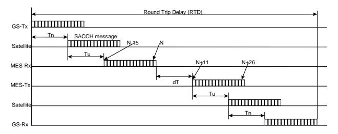
Figure D.3: Timing relationship for SACCH message round-trip transmission
