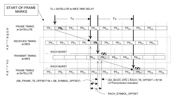
Figure 5.2: RACH burst timing
