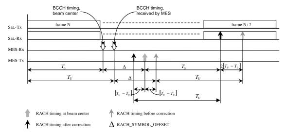
Figure 5.1: Initial timing synchronization process
