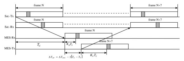
Figure 5.3: Frame and burst timing on the satellite and the MES
