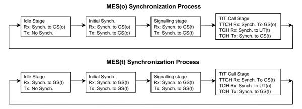
Figure 8.1: MES synchronization process for TtT call
