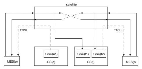
Figure 8.5: Transmission path during the TtT call
