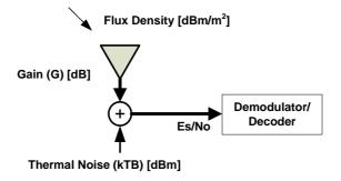
Figure 7.1: Radiated Sensitivity, G/T, and Es/No
