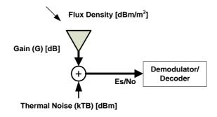
Figure 7.1: Radiated Sensitivity, G/T, and Es/No
