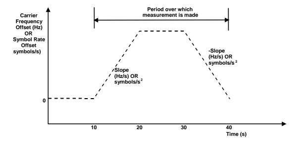
Figure 5.2: Frequency and symbol rate offset profile
