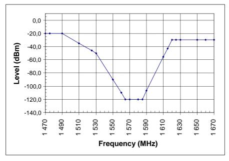
Figure 8.1: Out-of-band interference mask
