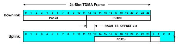
Figure 9.2: A RACH TS OFFSET example when PC12d and PC12u is used
