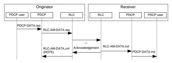
Figure 6: PDCP Data Transfer Over Acknowledged Mode RLC
