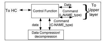
Figure D.1: V.44 Data Compression Functional Blocks
