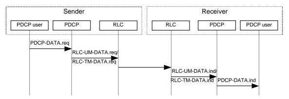
Figure 7: PDCP Data Transfer Over Unacknowledged or Transparent Mode RLC
