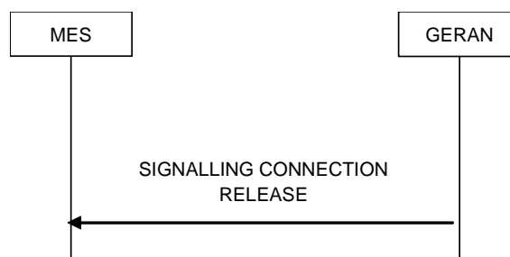
Figure 7.15.1.1.1: Signalling Connection Release procedure, normal case
