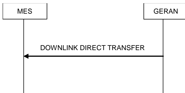
Figure 7.17.2.1: Downlink Direct transfer, normal flow
