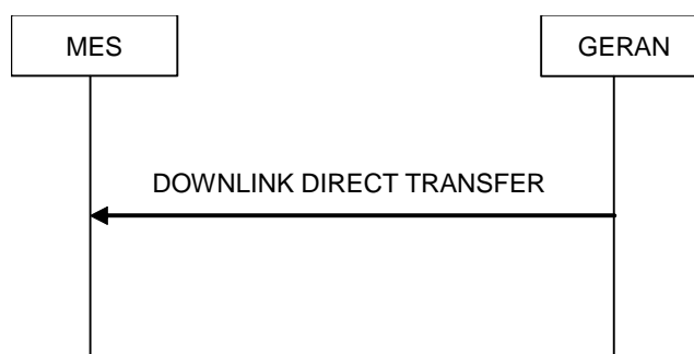
Figure 7.17.2.1: Downlink Direct transfer, normal flow
