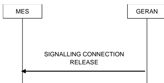
Figure 7.15.1.1.1: Signalling Connection Release procedure, normal case
