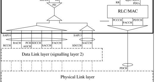
Figure 4.1: Protocol architecture of Radio Resource (RR) sublayer and RLC/MAC function
