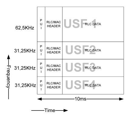
Figure 10.0c.4: Simultaneous transmissions on uplink
