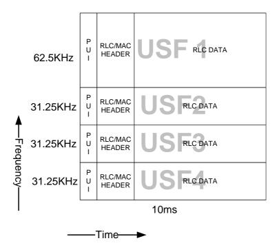
Figure 10.0c.4: Simultaneous transmissions on uplink
