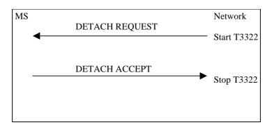
Figure 5.7.4: 2 GMR-1 3G 44.008: Network initiated GPRS detach procedure
