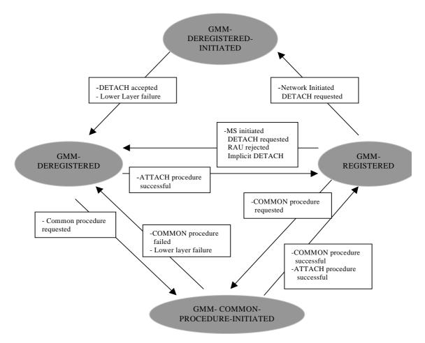
Figure 5.1b: GMM main states on the network side
