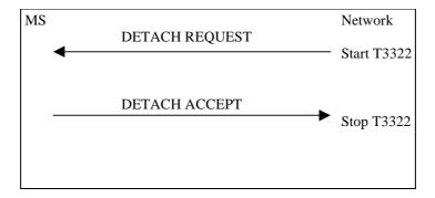
Figure 5.7.4: 2 GMR-1 3G 44.008: Network initiated GPRS detach procedure
