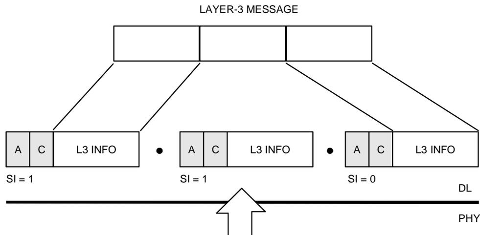
Figure 8.2: L3 message reassembling
