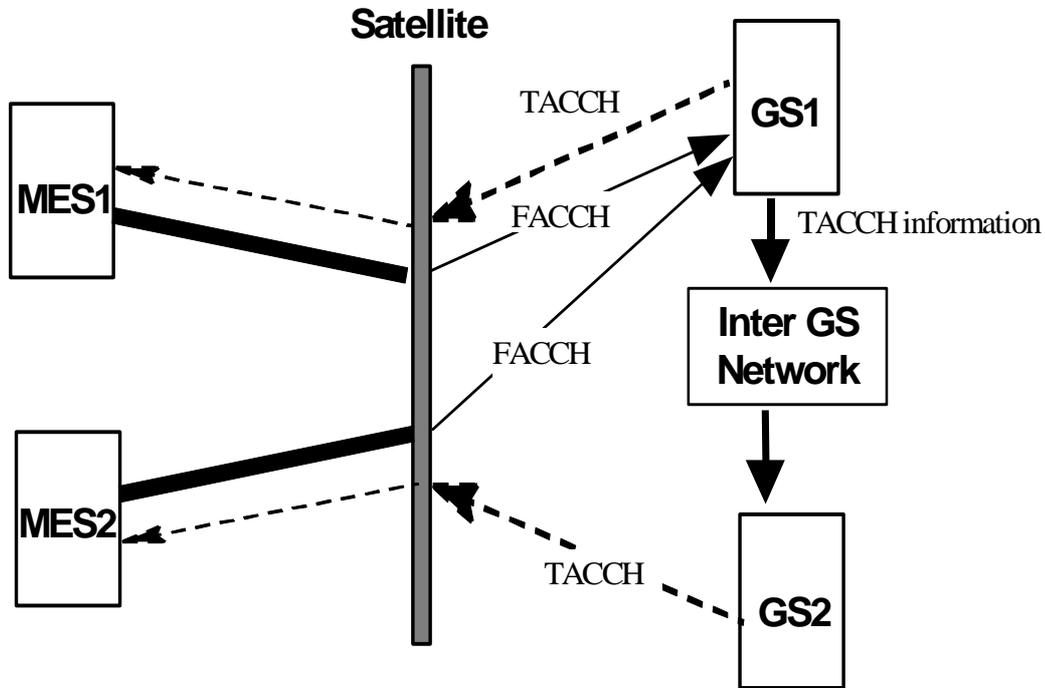
Figure 8.5: TtT call using two GSs
