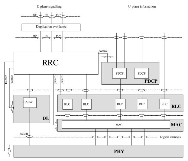
Figure 10: Radio Interface protocol architecture
