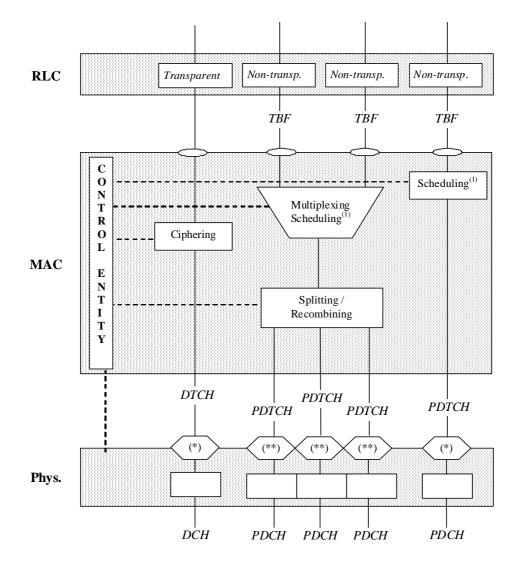
(\*): Such a SAP is created, re-configured and released by RRC User plane data (\*\*): Such a SAP is created, re-configured and released by MAC Control plane data (1): The scheduling function in this figure includes multiplexing user and control plane data and appending a MAC (possibly combined RLC/MAC) header to the MAC SDU.
