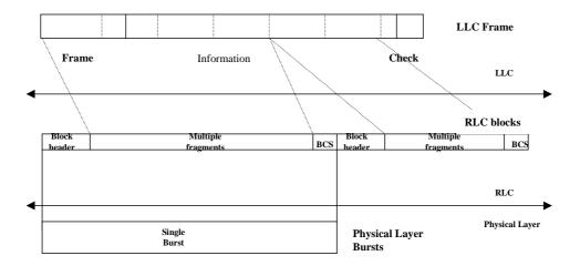
Figure 6: Transmission and reception data flow for GMPRS-1
