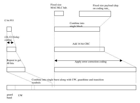
Figure 5: Radio block structure for MCS-1 to MCS-3
