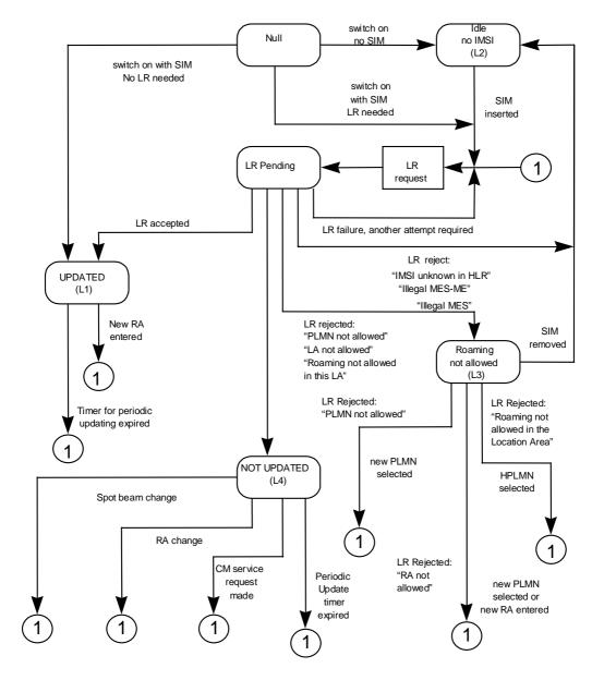
NOTE: Whenever the MES goes to connected mode and then returns to Idle mode again, the MES selects the appropriate state.
