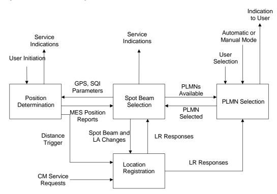
Figure 6.1: Four processes of idle mode
