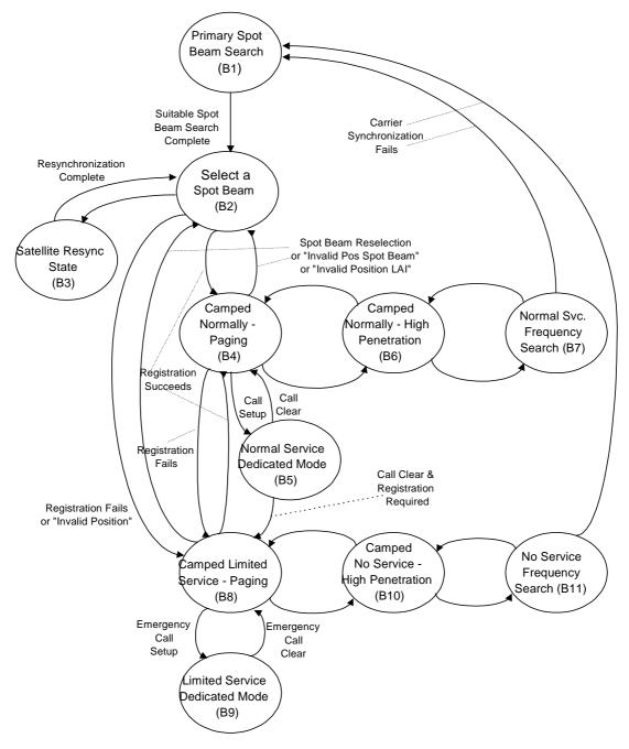
Figure 6.2: Spot beam selection process
