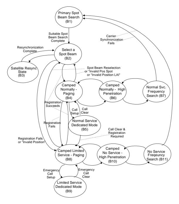
Figure 6.2: Spot beam selection process
