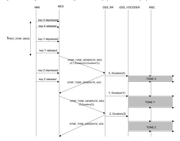
Figure 6.1: Call flow representation of the MES-to-PSTN DTMF transport for the GMR-1 system
