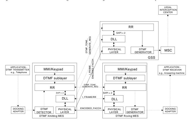
Figure 6.3: Functional block diagram of DTMF handling between two MESs in the GMR-1 system
