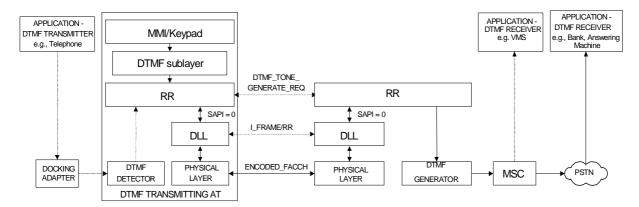
Figure 6.2: Functional block diagram of DTMF handling in the MES-to-PSTN direction in the GMR-1 system
