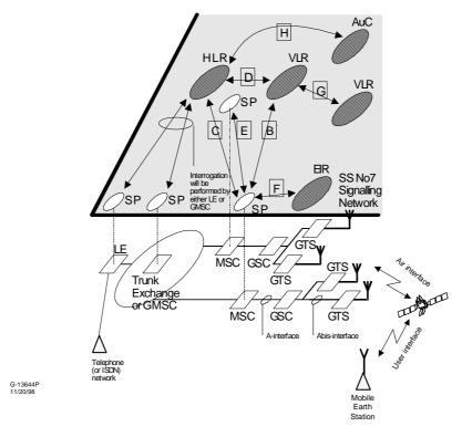
GSC Gateway Station Controller GTS Gateway Transceiver Station
