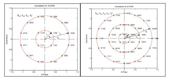
Figure 14: Signal constellations for 16 APSK and 32 APSK
