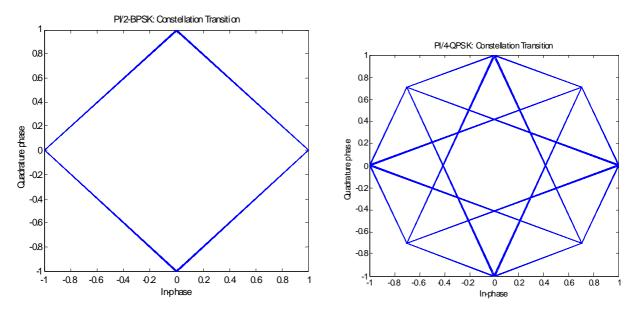
Figure 13: Signal constellations for  $\pi/2$ -BPSK and  $\pi/4$ -QPSK
