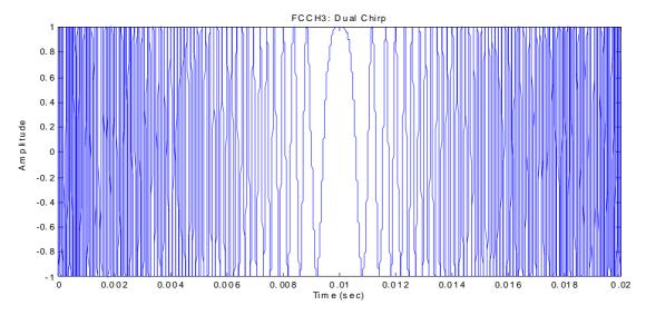
Figure 12: Dual chirp waveform
