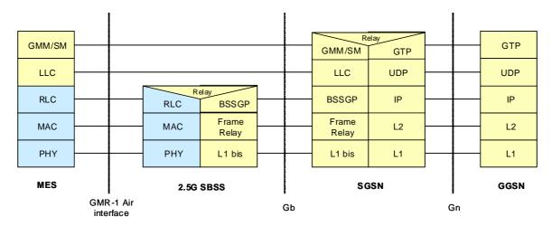
Figure 4: Protocol architecture for control plane (Gb interface)
