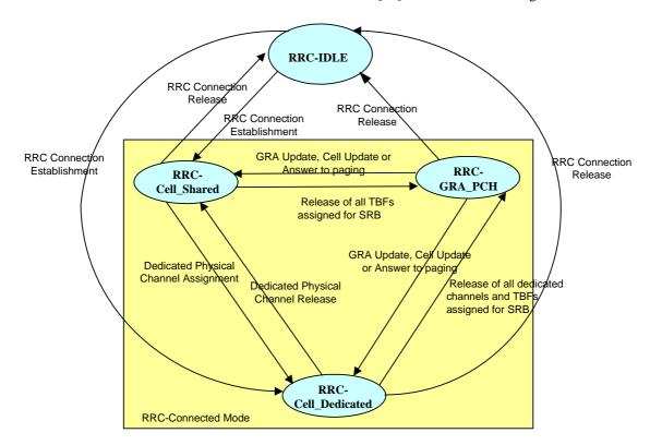
Figure 20: Radio Resource Control (RRC) state model
