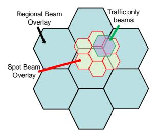
Figure 9: Example of a flexible satellite beam architecture
