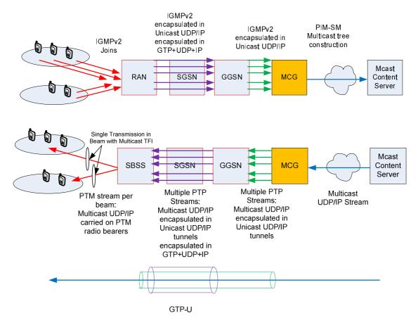
Figure 8: Efficient multicast implementation
