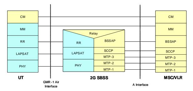
Figure 2: Protocol architecture for control plane (A interface)
