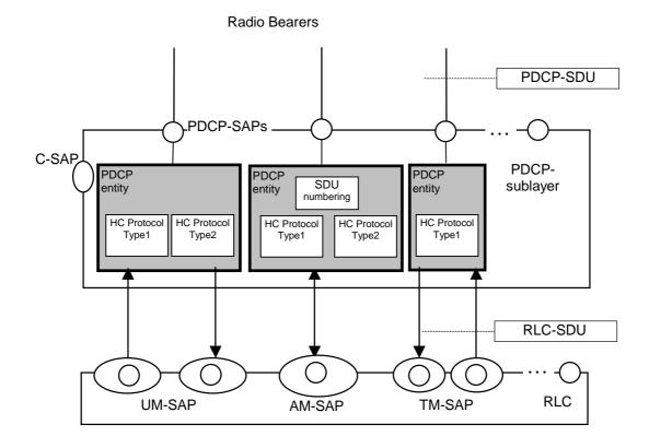
Figure 21: Packet Data Convergence Protocol (PDCP) structure
