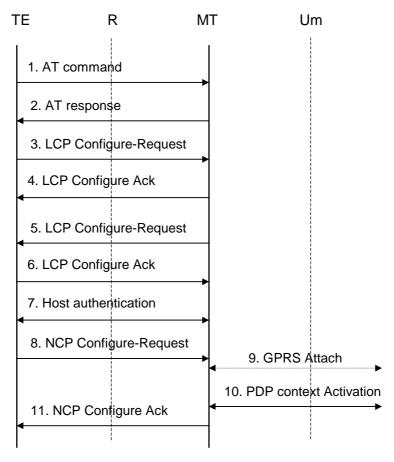
Figure 7: IP Over PPP Based Service
