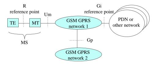
Figure 1:GPRS Access Interfaces and Reference Points
