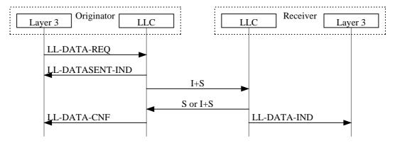
Figure 20: Transmitting and receiving I frames
