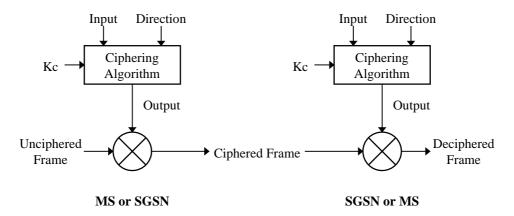
Figure A.1: GPRS ciphering environment
