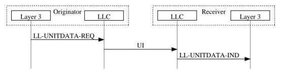
Figure 13: Unacknowledged information transmission
