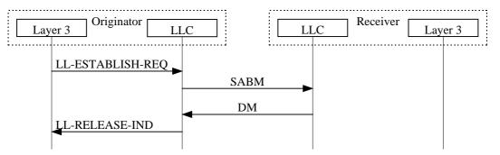
Figure 15: Layer 3-initiated ABM establishment procedure, unsuccessful
