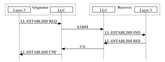
Figure 14: Layer 3-initiated ABM establishment procedure
