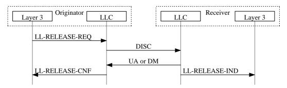
Figure 16: ABM release procedure
