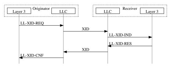
Figure 18: Layer 3 XID negotiation procedure
