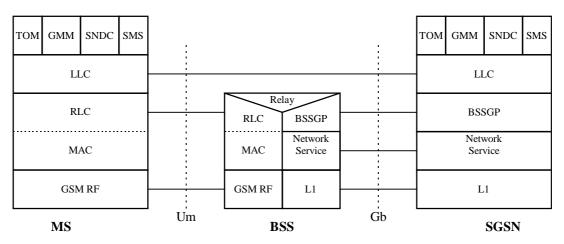
Figure 1: Protocol layering in GPRS
