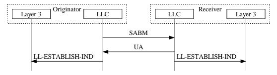
Figure 21: LLC-initiated ABM re-establishment procedure
