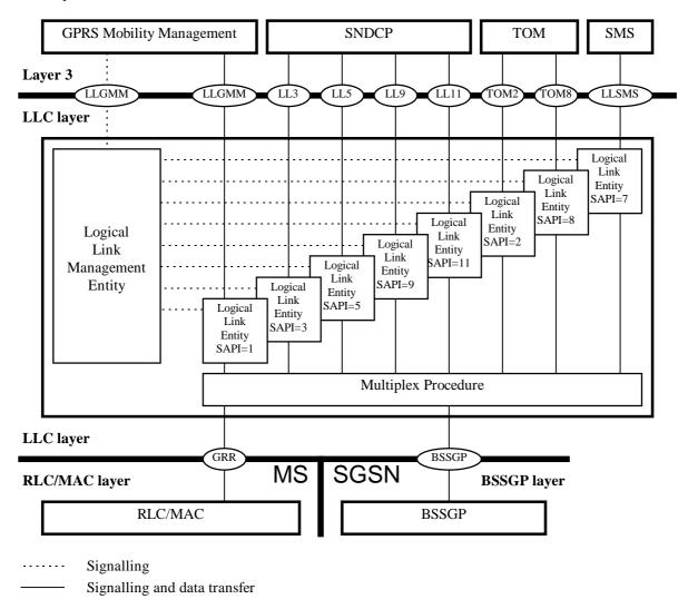
Figure 2: Functional model of the LLC layer
