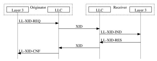
Figure 18: Layer 3 XID negotiation procedure
