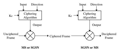
Figure A.1: GPRS ciphering environment
