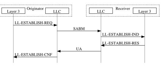
Figure 14: Layer 3-initiated ABM establishment procedure
