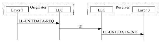
Figure 13: Unacknowledged information transmission
