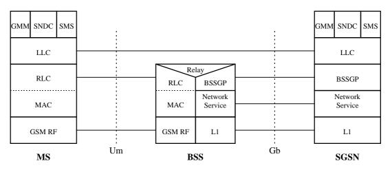
Figure 1: Protocol layering in GPRS
