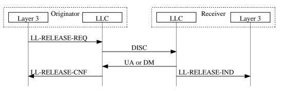
Figure 16: ABM release procedure
