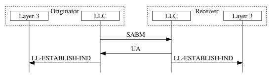
Figure 21: LLC-initiated ABM re-establishment procedure
