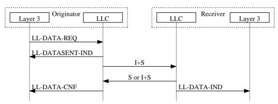
Figure 20: Transmitting and receiving I frames
