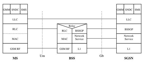
Figure 1: Protocol layering in GPRS
