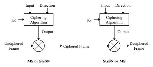
Figure A.1: GPRS ciphering environment
