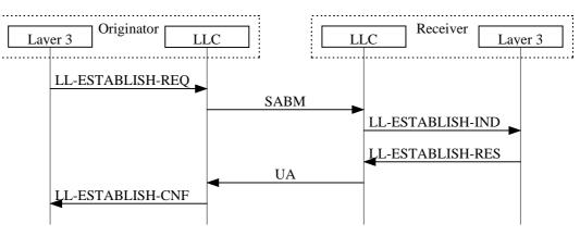
Figure 14: Layer 3-initiated ABM establishment procedure
