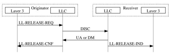
Figure 16: ABM release procedure
